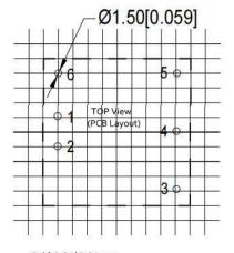
Grid:2.54\*2.54mm Unit:mm[inch] Pin tolerance:±0.10[±0.004] General tolerance:±0.50[±0.020]
