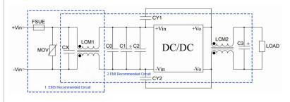
Note: Part 1 in the figure is for EMS testing, and part 2 in the figure is for EMI filtering, which can be adjusted according to the situation.
